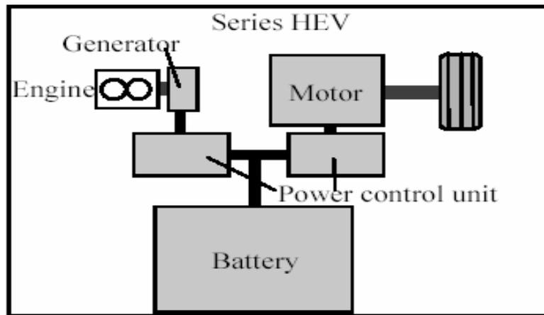
**Figure 1: Schematics of Series Hybrid Electric Vehicle [9]**
