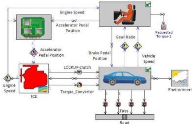
Figure 6. Conventional power plant model[8]
